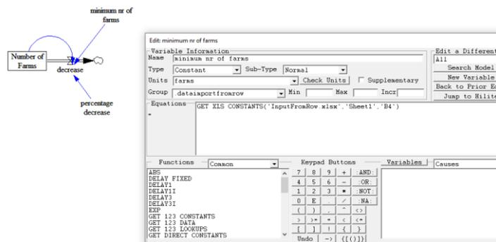
Figure 4 Tutorial example model demonstrating how to import a model parameter into the model.
