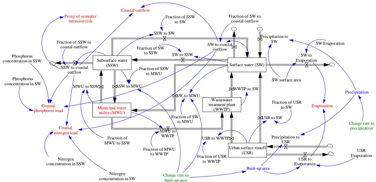
Figure 33: Stock-flow model structure for water availability for urban and tourism sector and their interactions with inland and coastal natural sub-systems. The main input and output variables are shown in blue and red, respectively. Change driving variables are shown in green in relation to hydro-climatic and land use changes.
