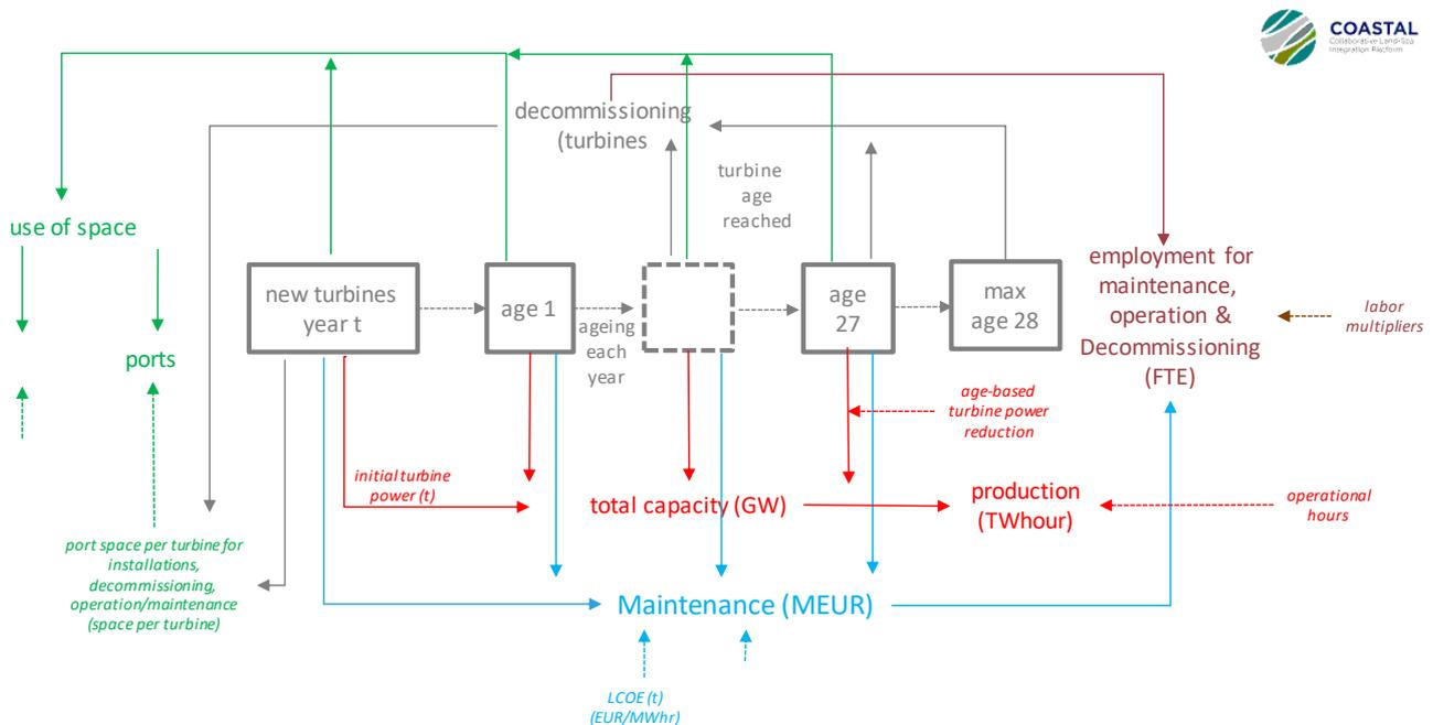
Figure 16 Port and Energy model focusing on the logistics and economic impacts of decommissioning offshore wind turbines (see deliverable D14).
