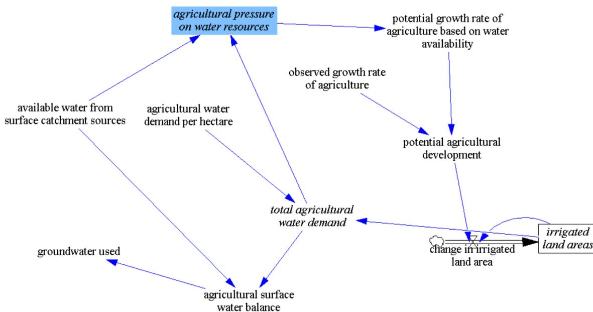
Figure 1. Overview of the generic model construct related to agricultural pressures on water resources and development of irrigated land areas.
