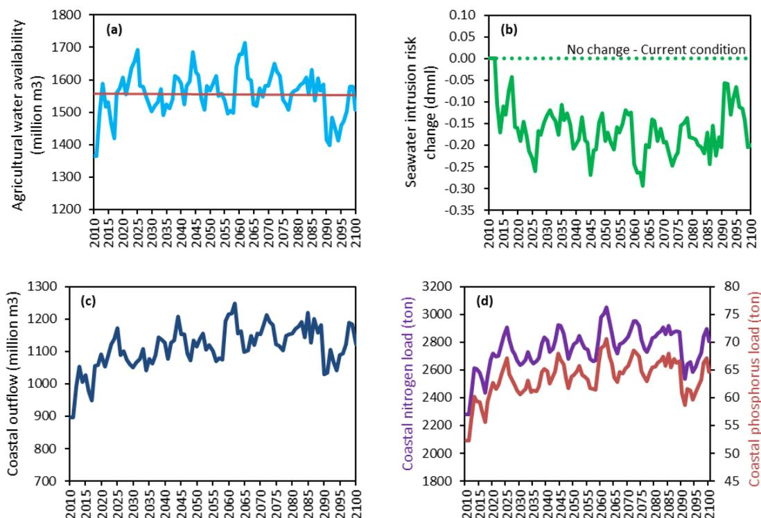
Figure 31: Demonstration results of the generic model construct for agricultural water availability under RCP4.5 and SSP1 change scenarios in MAL3: (a) agricultural water availability, (b) seawater intrusion risk, (c) coastal outflow, and (d) coastal nutrient loads.
