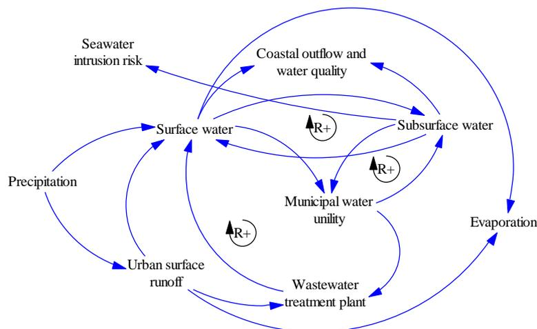
Figure 32: Interactions and feedback structures involved between inland and coastal natural sub-systems and urban and tourism sectors in MAL3. The reinforcing feedback loops are shown with the clockwise circles.
