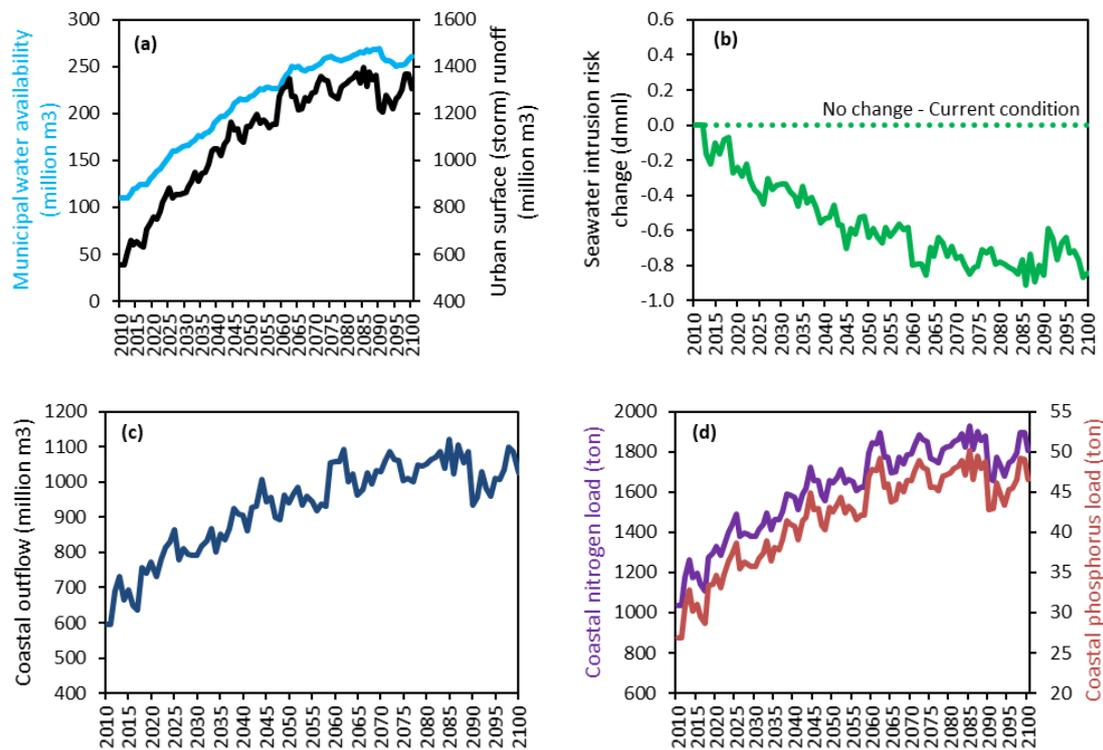
Figure 35: Demonstration results of the generic model construct for water availability for urban and tourism sector under RCP4.5 and SSP1 change scenarios in MAL3: (a) municipal water availability and urban storm water, (b) seawater intrusion risk, (c) coastal outflow, and (d) coastal nutrient loads.
