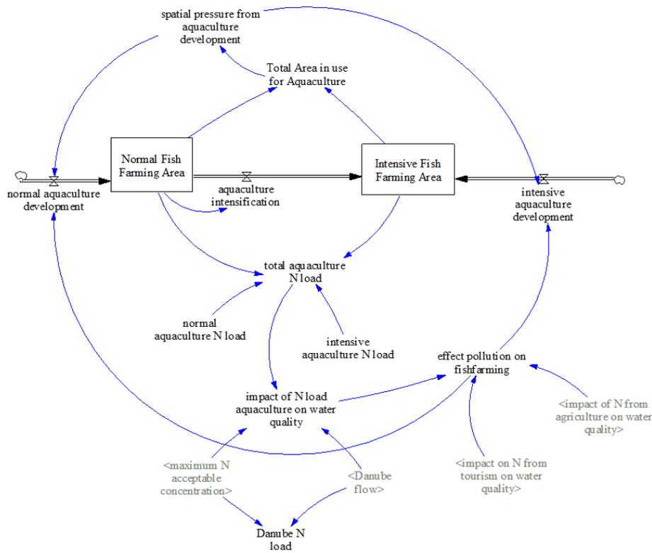
Figure 3.5.2.1. Overview of the generic model related to fish farming pressures on water quality
