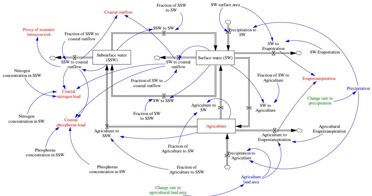
Figure 29: Stock-flow model structure for water availability for agriculture sector and its interactions with inland and coastal natural sub-systems. The main input and output variables are shown in blue and red, respectively. Change driving variables are shown in green in relation to hydro-climatic and land use changes.
