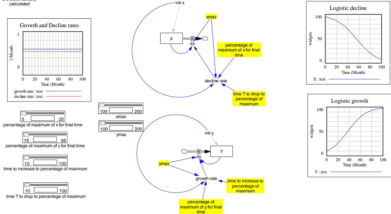
Figure 9 Automatic calculation of growth and decline rates from target values and time to reach these.
