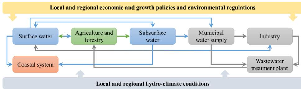
Figure 27: Main feedback loops involved in the integrated system dynamics (SD) model for MAL3. The colour of interactions is assigned based on the box colour of the influencing system component (de Kok et al., 2021).
