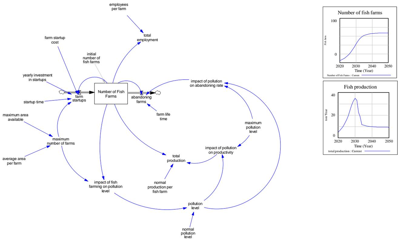
Figure 13 Generic structure for starting up a new sector, with fish farming as an example.
