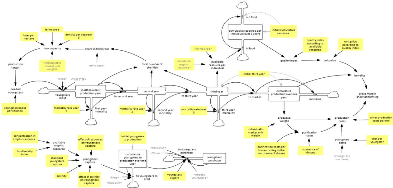
Figure 39: Generic SD shellfish farming model. Inputs are in yellow.
