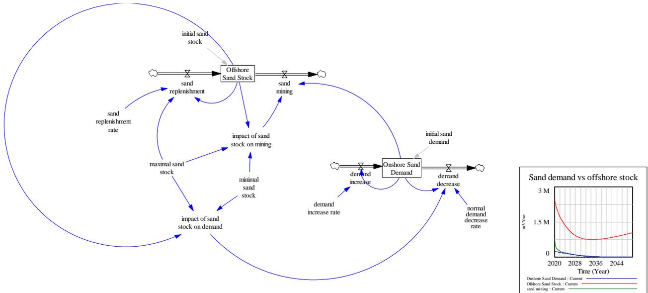
Figure 24 Model construct for offshore sand mining with interaction of demand, resource renewal and resource use.
