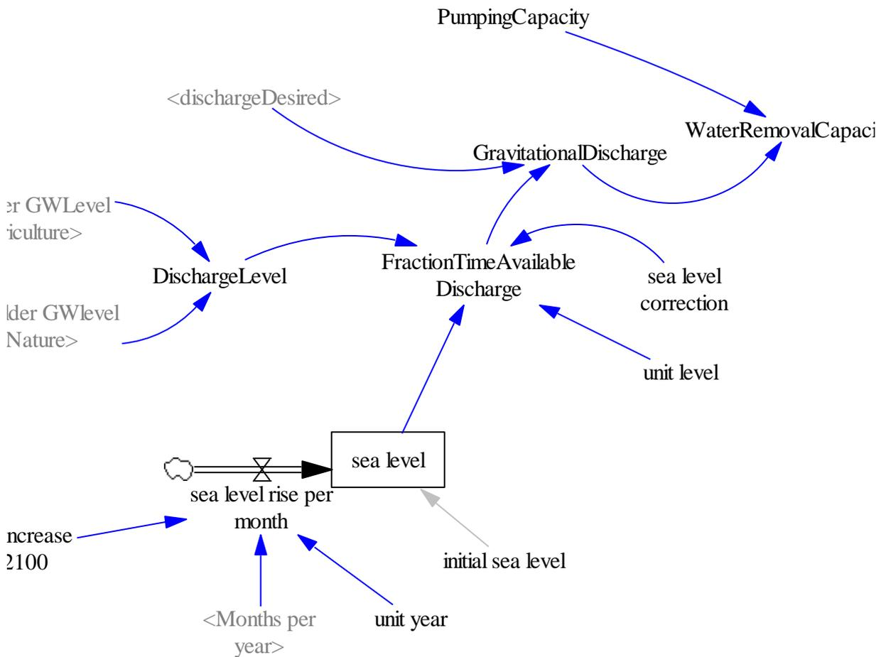
Figure 19 Model construct for the impact of sealevel rise on the operational window for discharging water to the sea as an strategy for water management.
